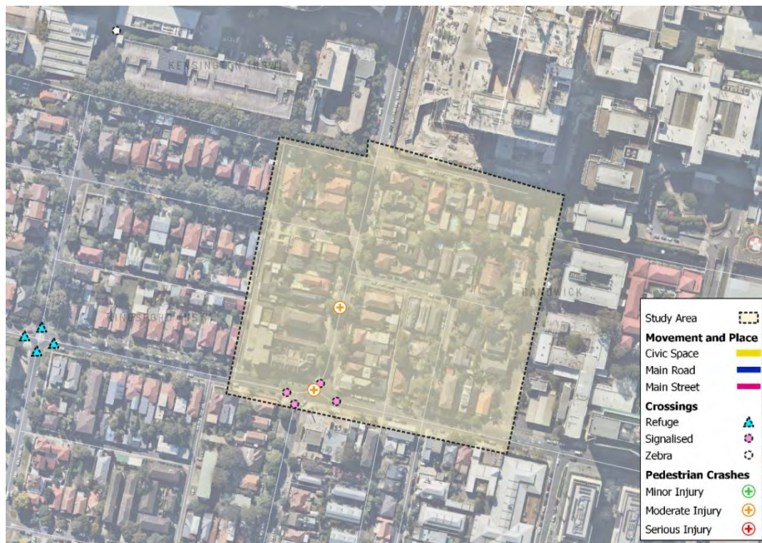
Figure 8.5: Magill Street – Street Classifications, Crossing Facilities and Pedestrian Crashes
