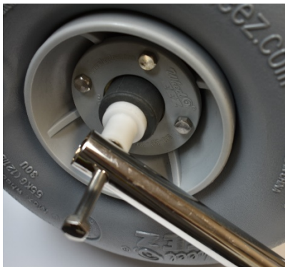
Center wheel between caster forks and install bolt
