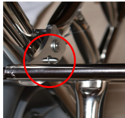
Locking bar and pin engaged.
