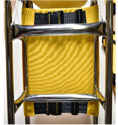
Install seat bottom pad and attach buckles.
