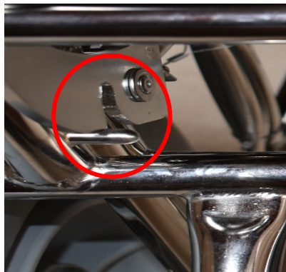
Locking bar and pin disengaged.
