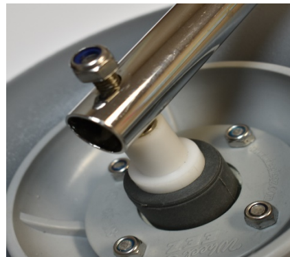
Install and tighten lock nut
