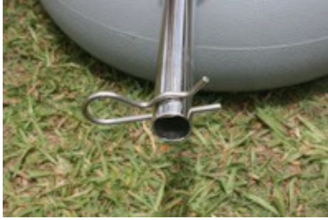
Remove Hitch Pin from axle.
