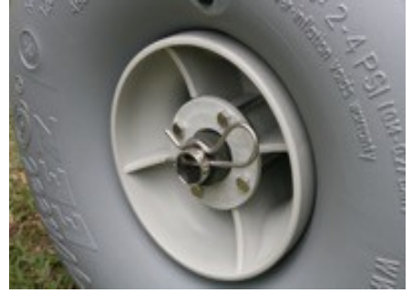
Reinstall Hitch Pin to retain wheels.
