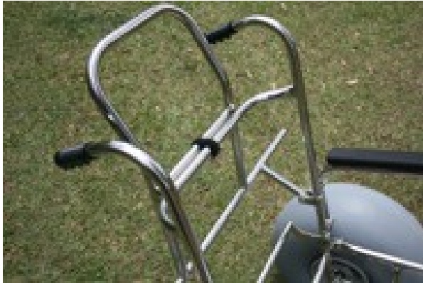
Anti-tip/ parking brake in stowed position.
