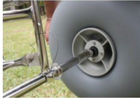
Install wheel onto axle.
