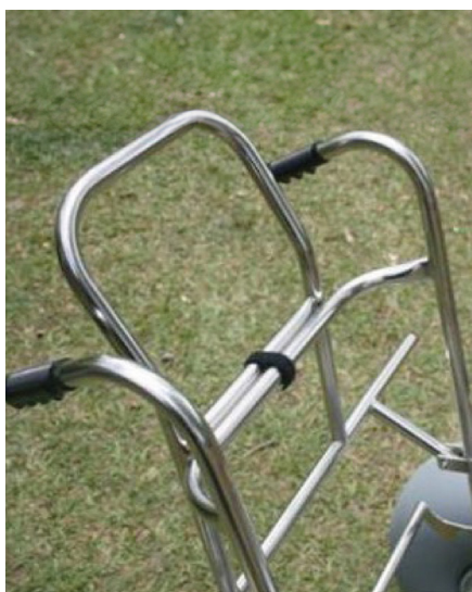
Figure 1 - The anti-tip mechanism/ parking brake is found at the rear of the chair below the hand rail. When the anti-tip mechanism is not in use it is attached with Velcro to the top crossbar between the push handles.
