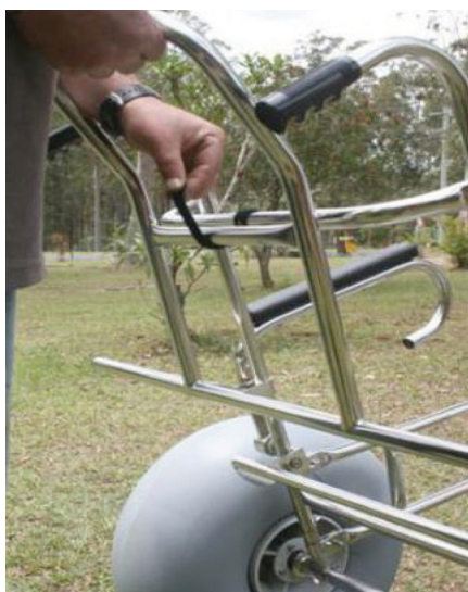
Figure 2 - To apply the park brake/ anti-tip bar, unhook the Velcro strap from the cross bar.
