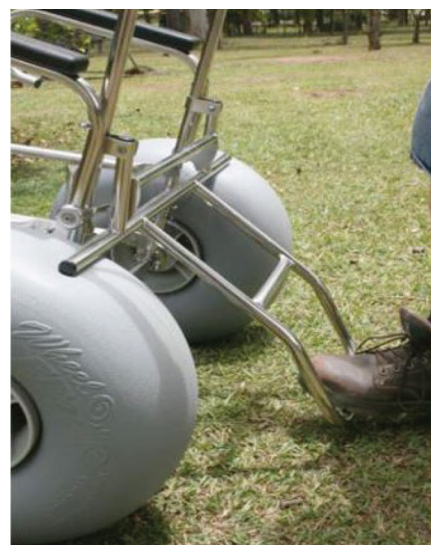
Figure 3 - Swing the bar down and place foot on middle of the bar and push against tyres until locking bar is engaged.
